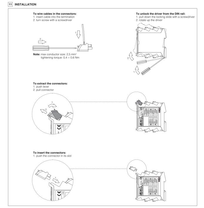
Note: all connectors are supplied with a mechanical coding. This feature ensures a unique insertion of each connector in the own slot. (e.g. connector A can not be inserted into connector slot of B,D,E,F)
