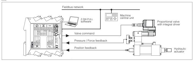
Note: block diagram example for alternated position/force control, with fieldbus interface
