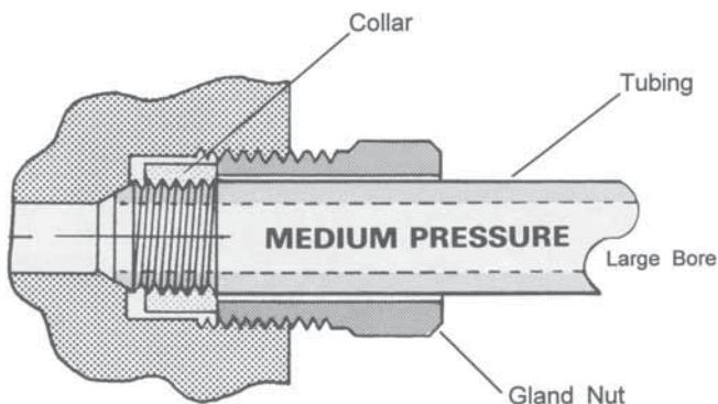
**Medium Pressure** is a 58/60° coned and threaded tubing design.
