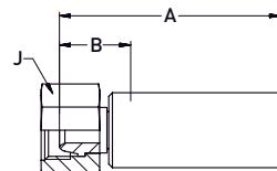
**MATERIAL** Carbon steel, zinc plated (shell and nut)
