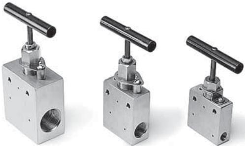
Developed to assure safe and easy plumbing through 60,000 psi. These needle valves are engineered to the highest standards of repeatable quality. The medium pressure valves are designed with a compact cone-and-threaded connection which permits the larger bore sizes and increased flow rates common in this pressure class. The high pressure valves also use a coned-and-threaded connection which accommodates the high pressures common in these applications.
