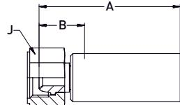
**MATERIAL** Carbon steel, zinc plated (shell and nut)
