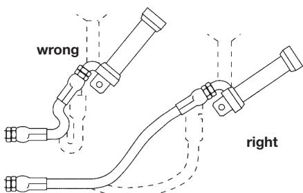
When hose assembly is installed in a flexing application, remember that metal hose fittings are not part of the flexible portion.
