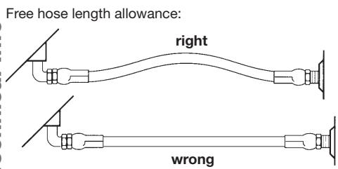
Pressure can change hose in length by as much as  $\pm 2\%$ . This must be considered when cutting hose to appropriate length.
