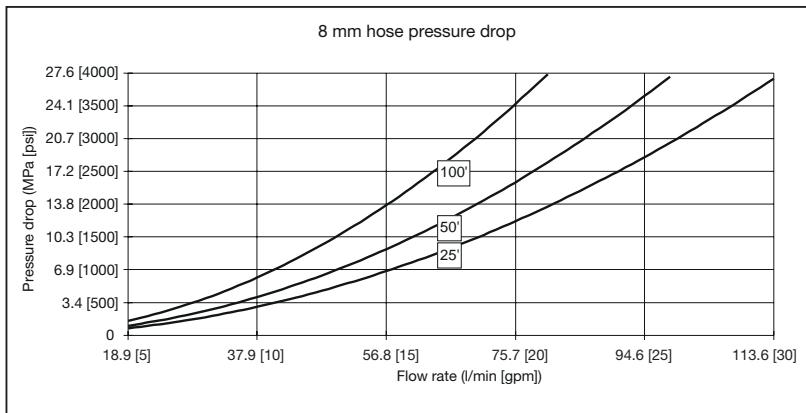
Results obtained from actual pressure drop tests, pumping water through hose assemblies with normal end fittings.
