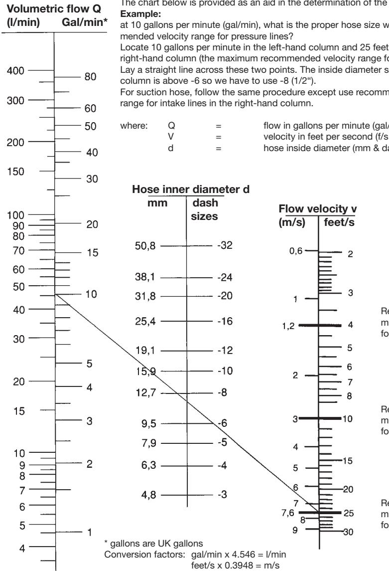
\* Recommended velocities are according to hydraulic fluids of maximum viscosity 315 S.S.U. at 38 °C working at roomtemperature within 18 ° and 68 °C.
