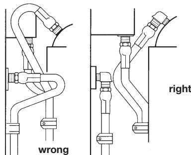
Use elbows or adaptors as necessary to eliminate excess hose length and to ensure neater installation and easier maintenance.
