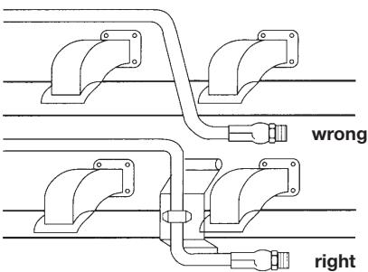
Avoid installing hose assemblies close to heat sources. However, if this should be required, insulate hose.
