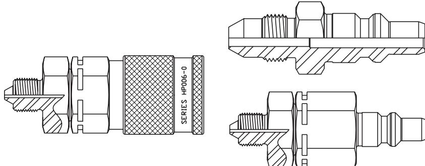
A versatile connecting device that permits easy and rapid joining of hose assemblies to your system. Each coupling is assembled and pressure tested to at least 5,000 psi above its maximum rated working pressure. Couplings with check-valve can withstand the full working pressure in the disconnected condition.
