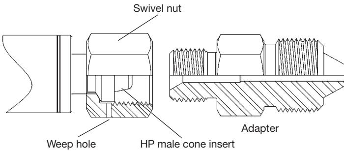
The Type "M" Swivel End Fitting is a swivel nut fitting with a 58° male cone nipple.
