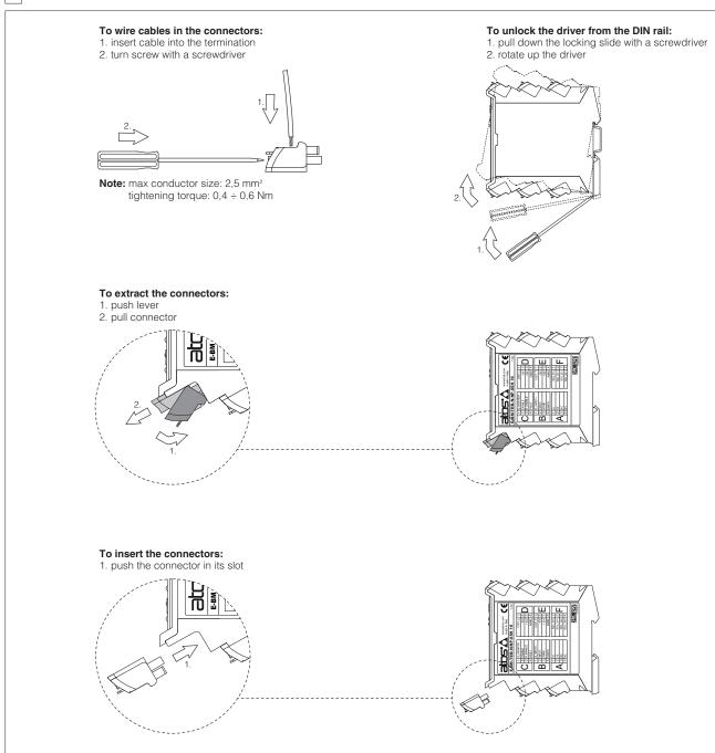
**Note:** all connectors are supplied with a mechanical coding. This feature ensures a unique insertion of each connector in the own slot. (e.g. connector A can not be inserted into connector slot of B,C,D,E,F)
